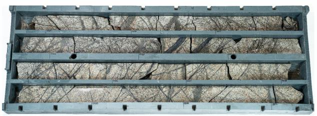
**Figure 3:** Drill core (HQ) from CPW0002DD showing similar style and intensity of stockwork quartz-sulphide veining as per CPW0001DD. The core in this photo is from 679.40 m – 683.06 m depth (2229' – 2241') part of logged interval 673.61 m – 694.03 m (2210' – 2277') which contains visually estimated 4% pyrite, 1% chalcopyrite and 0.4% molybdenite and 8 volume % quartz-sulphide veining.
