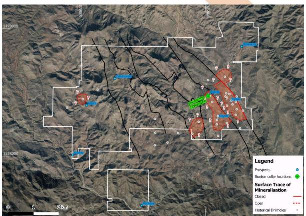
**Figure 4:** Location of Buxton drillholes CPW0001DD and CPW0002D within defined mineralisation from drilling by historic explorers. Mineralisation is open in most directions and depth. Interpreted extensional structures offset mineralisation and control the development of high-grade supergene chalcocite mineralisation. Current lode mining claims and exploration permits outlined in white (external perimeter of tenement holdings shown only).
