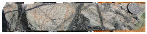
**Figure 1:** Porphyry-style alteration, veining and mineralisation in CPW0001DD at 594.66m. This section of HQ core is part of assayed interval 594.06 – 595.88 which returned 3936 ppm Cu and 745 ppm Mo for 0.92 % CuEq<sup>1</sup>.
