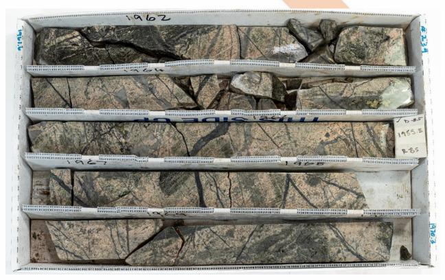
**Figure 2:** Drill core tray (HQ) from CPW0001DD showing high intensity of stockwork quartz-sulphide veining overpriting felsic gneiss and mafic schists. The upper section of HQ core in this photo is part of assayed interval 597.71 m – 599.54 m (1961' – 1967') which returned 7057 ppm Cu and 1295 ppm Mo for 1.62% CuEq<sup>3</sup>. The lower section of core is part of assayed interval 599.54 m – 601.37 m (1967' – 1973') which returned 2690 ppm Cu and 1509 ppm Mo for 1.33% CuEq<sup>3</sup>.
