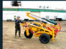
Compressed Air Blast Hole Rig
