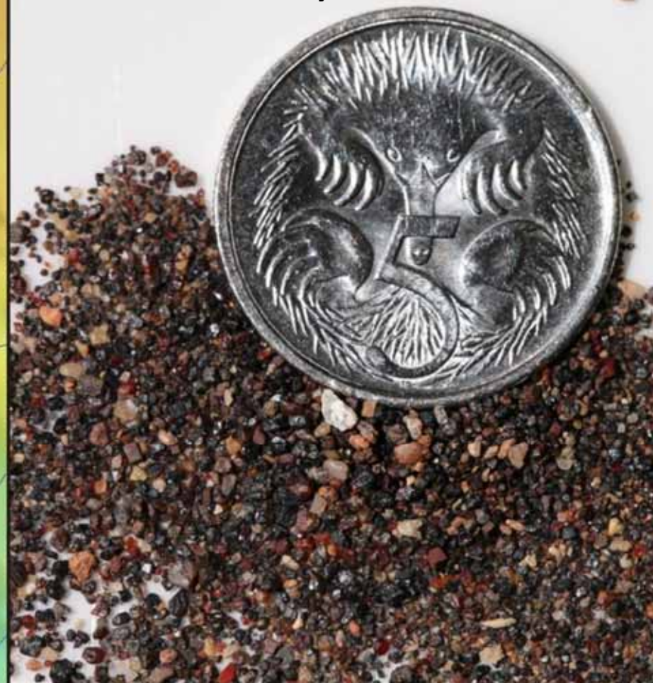
Cassiterite rich heavy mineral concentrate
