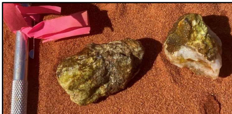
Figure 1: Reaper trend air core drill hole 20PTA0064 drill-chips from 66m showing ferruginous quartz-sericite veining and alteration within gold-bismuth mineralisation zone
