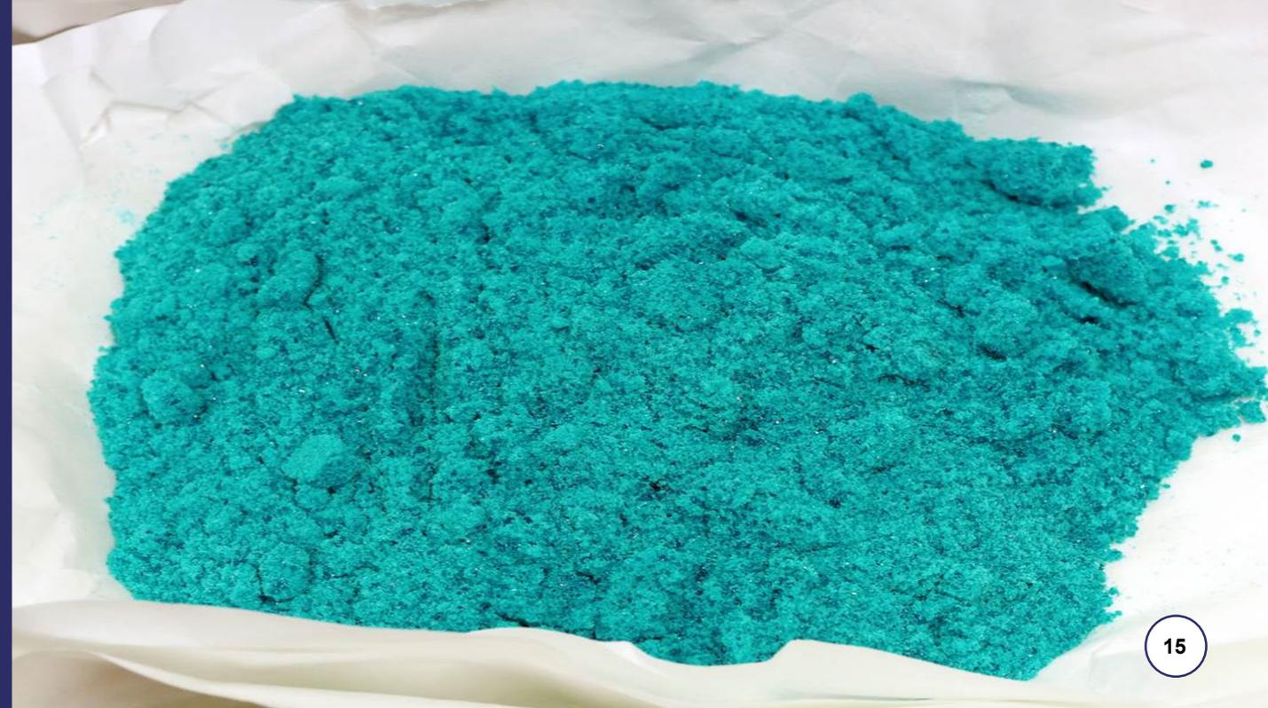
1) Photographs to the RHS are of the 1.6kg of nickel sulphate hexahydrate crystals produced in the metallurgical testwork. Photography by Karel Osten, Wood Plc
