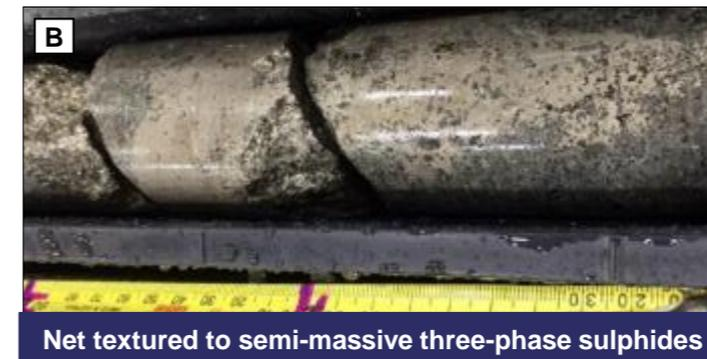
Net textured to semi-massive three-phase sulphides
