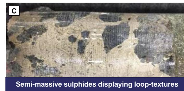
Semi-massive sulphides displaying loop-textures
