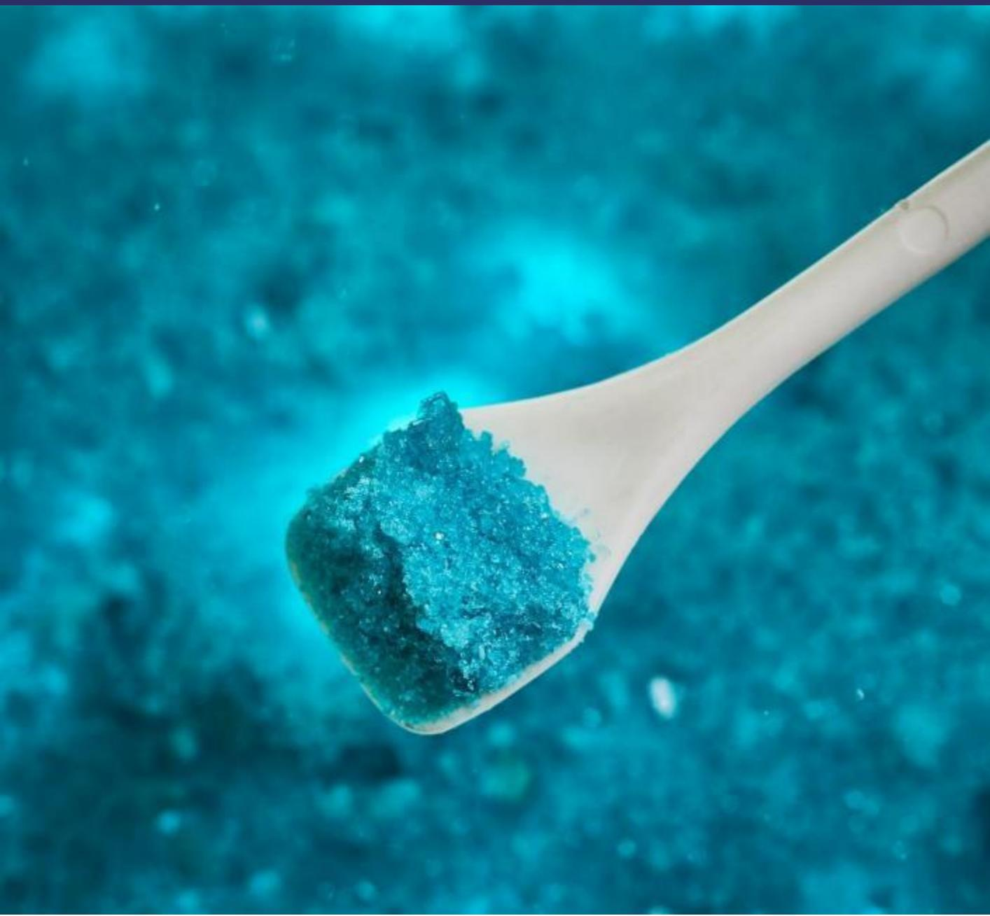
**Nickel sulphate is a key raw material within the cathode of modern lithium ion batteries**
