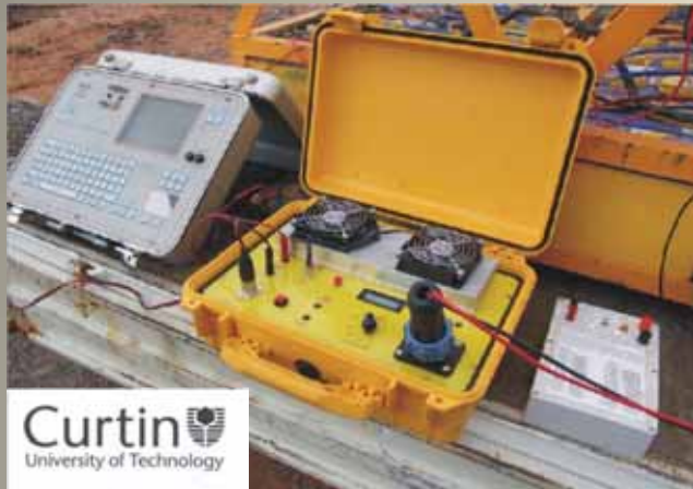
High powered TEM transmitter
