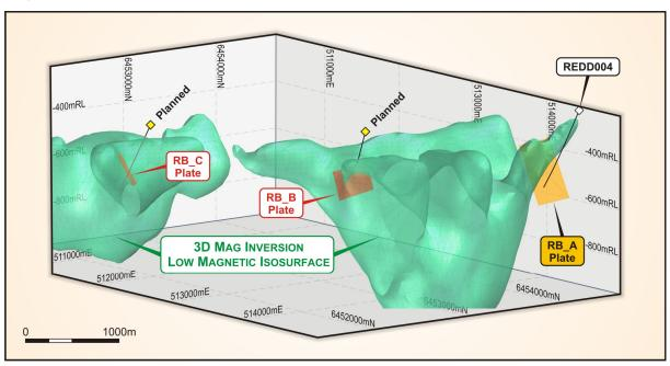
Figure 2: 3D view, looking northwest, of the targeted conductor plates RB\_B and RB\_C in relation to the low magnetic unit representing mafic intrusive bodies interpreted from the magnetic inversion<sup>1</sup>.
