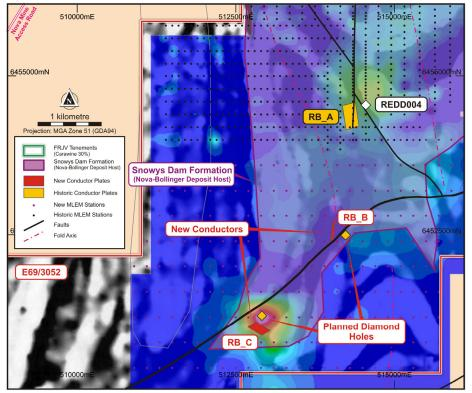
Figure 1: Red Bull conductor targets and planned hole locations (image is of late time MLEM channels overlying grayscale regional magnetics)<sup>1</sup>.
