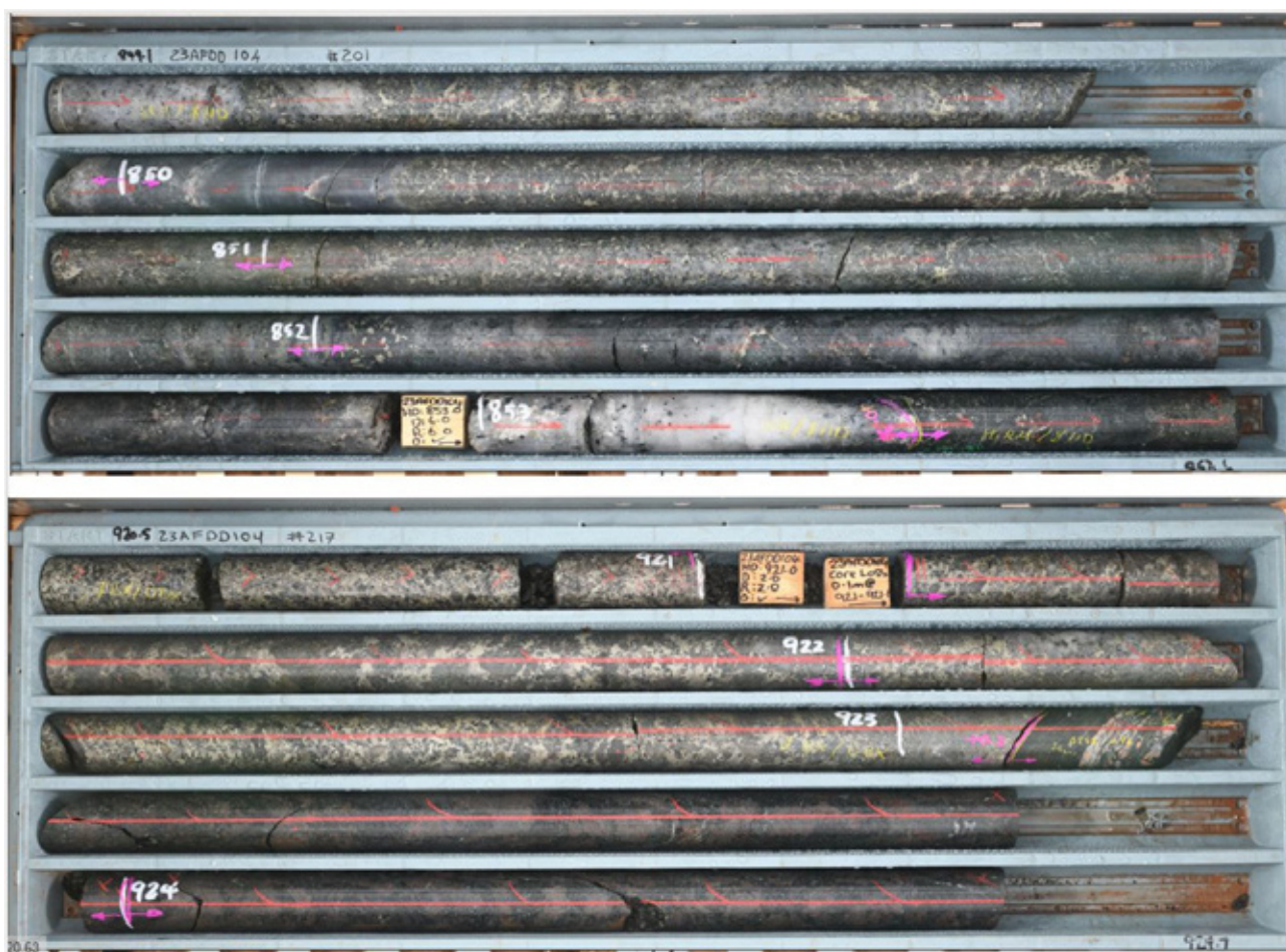
Figure 17: Pyrrhotite-chalcocopyrite-sphalerite sulphides in drill core from hole 23AFDD104
