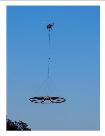
Figure 1: NRG helicopter undertaking AEM survey over E70/4688
