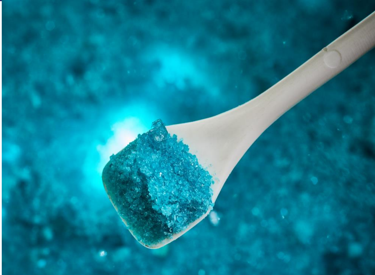
Battery grade nickel sulphate produced via the IGO Process
