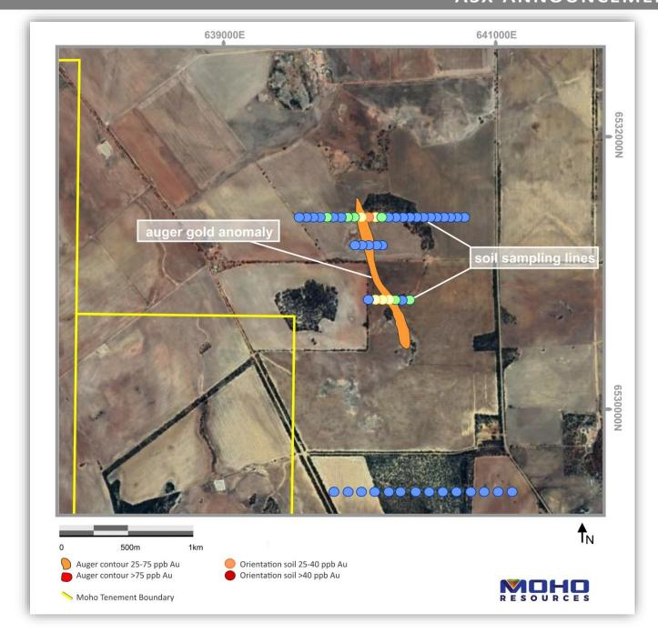
Figure 4: Locations of soil samples and gold auger anomalies at Golden Hind Prospect
