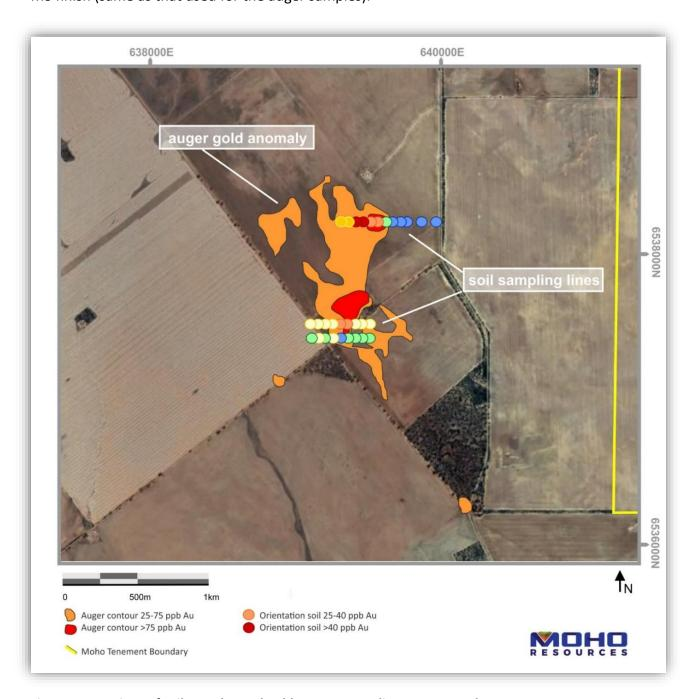
Figure 3: Locations of soil samples and gold auger anomalies at Crossroads Prospect
