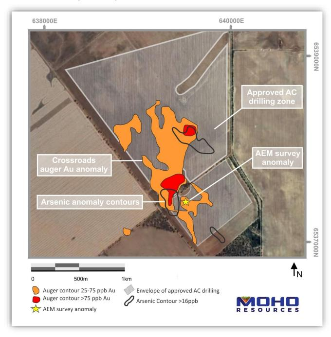
Figure 6: Program of Works-approved envelope for air core drill program over gold and arsenic auger anomalies and AEM anomaly at Crossroads Prospect
