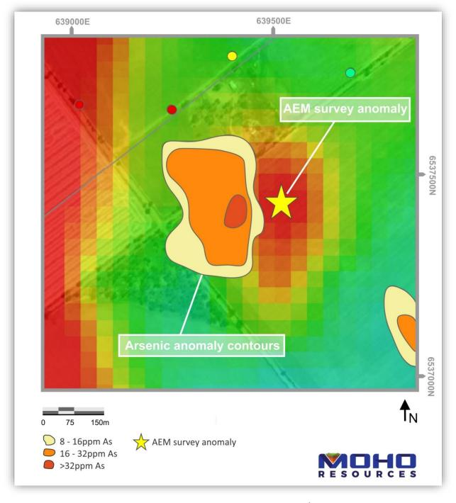
Figure 2: Coincident arsenic and AEM anomaly, Crossroads Prospect (processed Airborne EM data (channel 15) overlain on Google Earth image)
