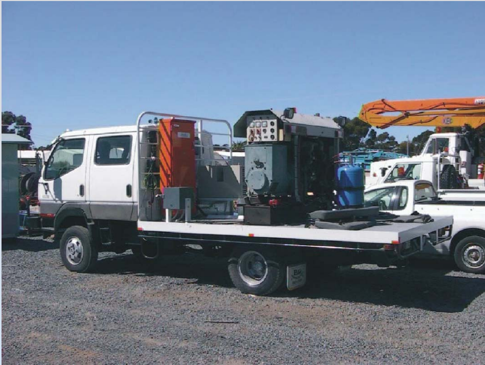
High powered TEM transmitter truck developed in conjunction with Curtin University
