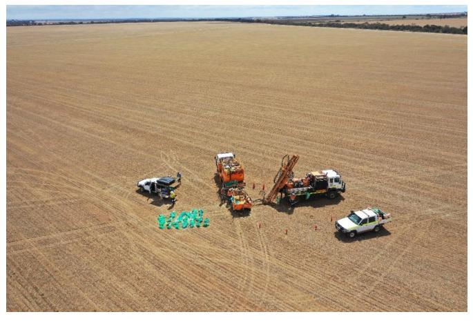
Figure 1: Air core drilling at Crossroads prospect March 2020 with 'Low Impact Rig', Burracoppin Gold Project
