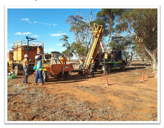
Figure 1: Aircore drilling at Crossroads prospect with 'Zero Impact Rig', Burracoppin Gold Project
