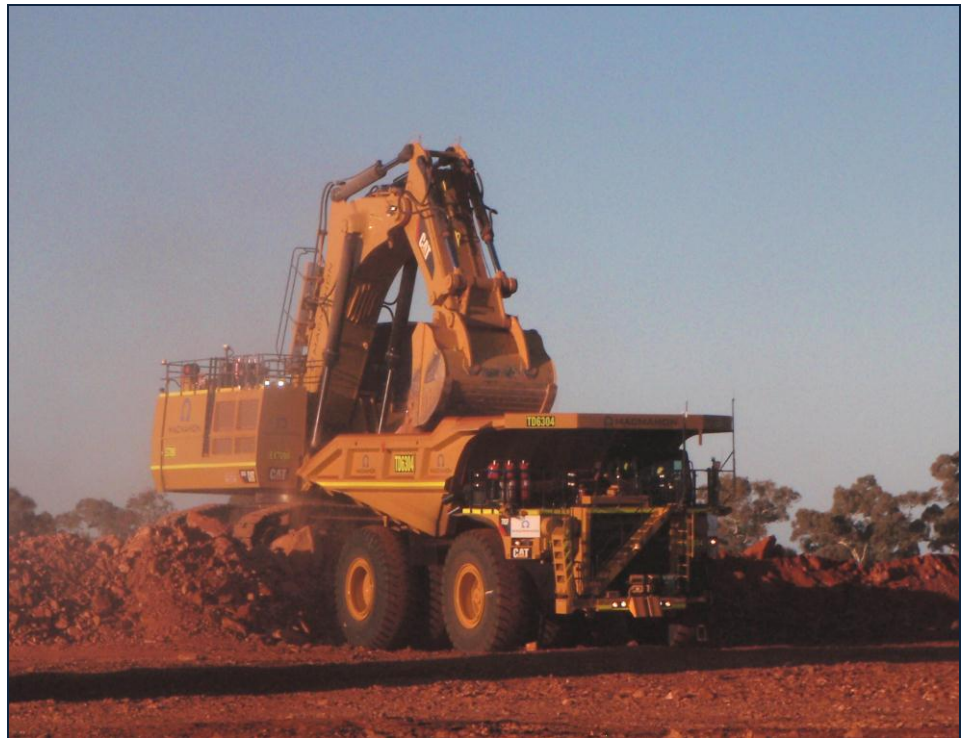
Photo 1: Commencement of mining, with pre-stripping of the Havana Pit. The recently assembled 400 tonne CAT 6040 excavator loads one of the 225 tonne payload CAT 793F dump trucks.
