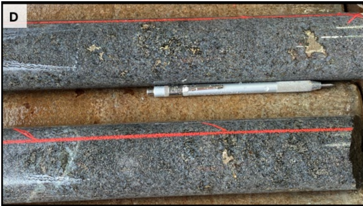
Figure 2 Coarse three-phase Po-Cp-Pn blebs and carbonate veinlets in gabbronorite at 464m in 21AFDD104.
