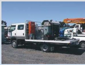
High powered TEM transmitter truck developed in conjunction with Curtin University
